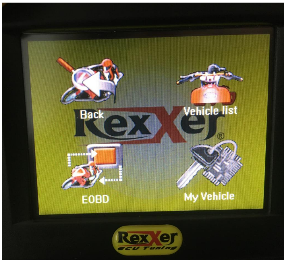
Figure 7: Menu item Diagnostic: For using the service-/diagnostic function select the item “my vehicle”. If your vehicle is not recognized, select the item “vehicle list” and choose your vehicle directly.
