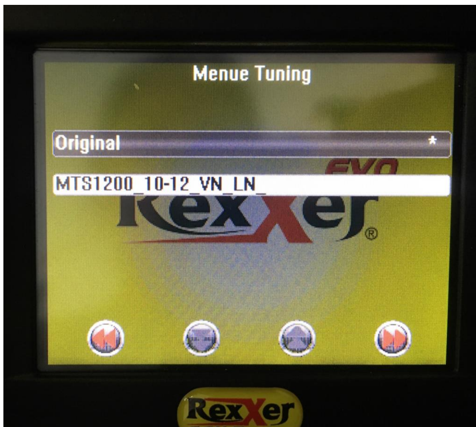
Figure 6: Menu Tuning: Here is every Mapping listed which is stored in the device memory. The marked (*) Mapping is currently in the ECU.
