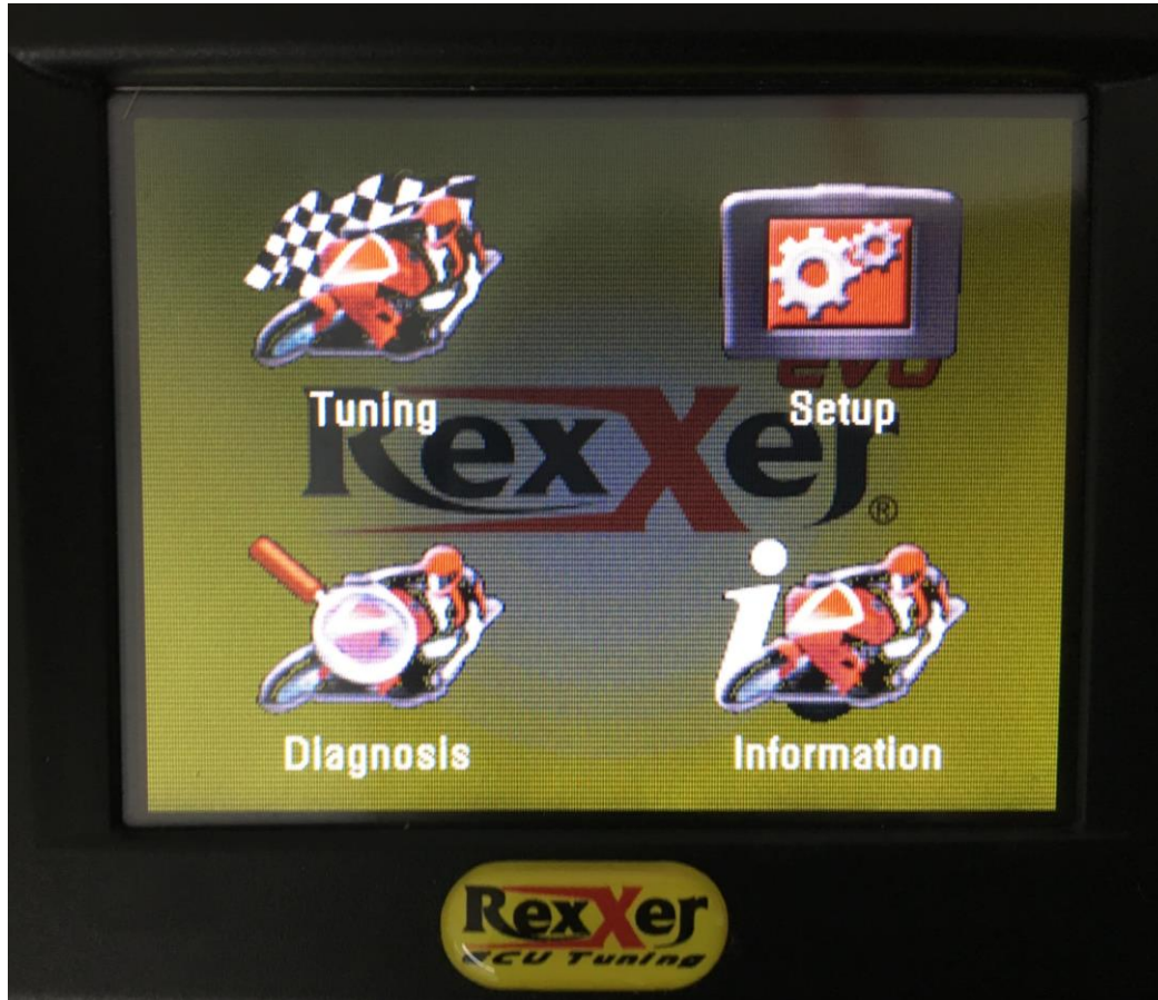
Figure 1: Main menu: By connection the RexXer EVO User with your motorcycle over OBD this main menu will be opened automatically.
